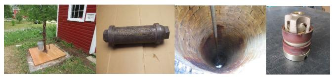
(From left to right) Our W. L. Davey pump / Pump cylinder attached to the pipe below the water level / 20' deep well with 6' of standing water and cream city brick lining / Mechanism which fits inside the cylinder and lifts the water with each stroke.
